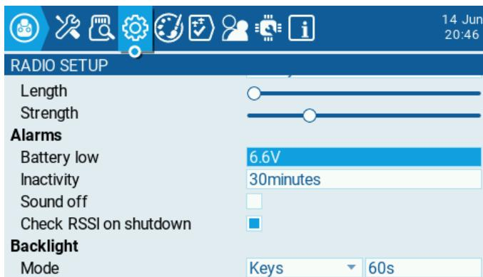
Under “Backlight”, set the way you’d like for the backlight to operate. If you set it to “ON”, the backlight is on all the time. If you change it to “Keys”, only the menu buttons will cause the backlight to come on, and then you can choose how long the backlight should stay on once activated.
