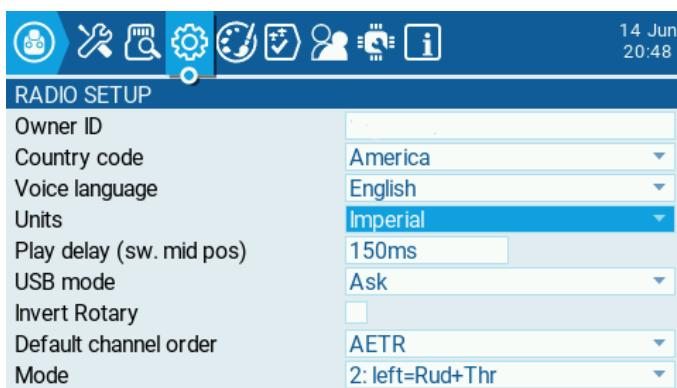
Set “USB mode” to “Ask” and it will ask you what it should do (access storage or work as a joystick controller) when USB is connected.
