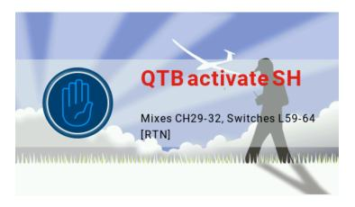
This is a notification that the Mixes, Logical Switches, and Custom Function that implement QTB have been installed and that the activation switch has been assigned – in this example SH, the momentary action switch on the TX16S. This will be the case for most radios, but there are 5 radio types that do not have an SH switch and 3 of those do not have a momentary action switch.
