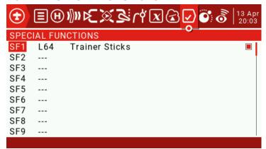
The simple one – L64 controls the Trainer mode. The install script will take over an existing Trainer Sticks line if one already exists. If not, it will put this line in the first unused slot of SPECIAL FUNCTIONS. You can move it anywhere you want after installation. If the install script erase function is used, this line will remain, but be disabled.
