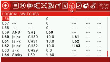
59 is ON when the conditions are met to turn trainer mode on.
